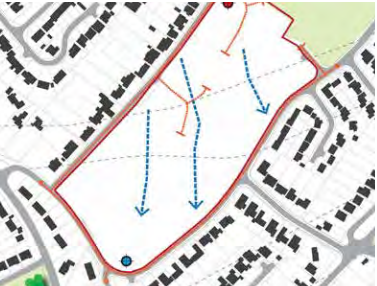
SuDS Constraints and Opportunities Diagram ● High point ➡ Direction of flows ● Low Point - - - - - Existing combined sewer
