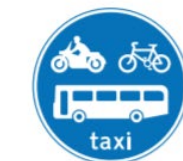
Figure 9-24 Diagram 953B (S3-2-35) Route for use by buses, pedal cycles, solo motor cycles and taxis only (Alternative types)
