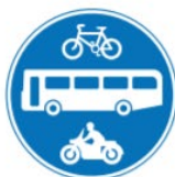
Figure 9-23 Diagram 953A (S3-2-34) Route for use by buses, pedal cycles and solo motor cycles only (Alternative types)
