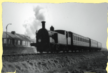
This train is an M7 tank, push pull set. It is running on the Brighton to Horsham line, adjacent to the A283 Old Shoreham Road and is approaching Shoreham toll bridge from the South.
