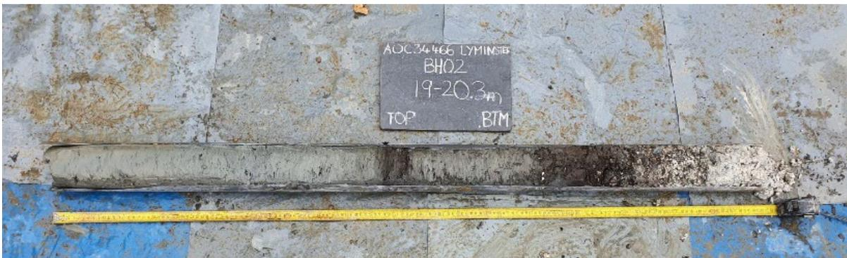
**ABOVE: A machine drives a borehole through the 'Black Ditch' sediment. BELOW: A borehole sample showing different layers from the Black Ditch.**
