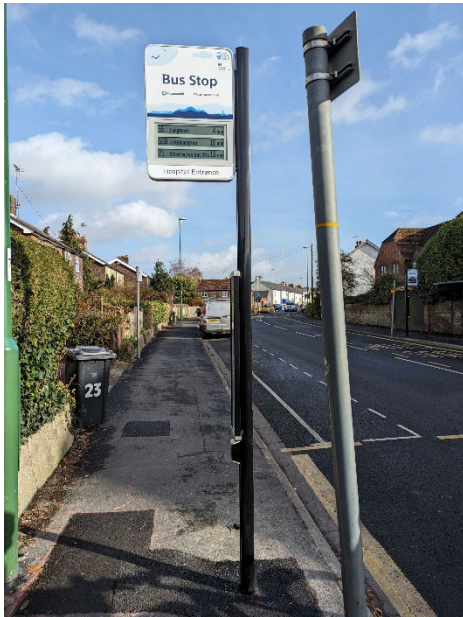
Image 1. RTPI Unit on bus stop post
