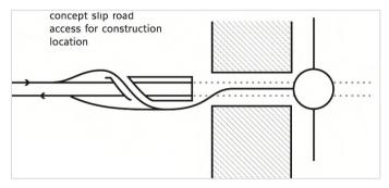
8.3.45 For the second concept it is most likely that some land-take will be required to enable slip roads to be provided, either to the north, south or both north and south; our figure illustrates a carriageway realignment to provide slip road access.
