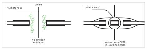
8.3.14 Whilst both the 'with junction' or 'no junction' would be likely to have an impact on the Centurion Way footway/cycleway, the 'no junction' green bridge configuration would provide an opportunity for a car/junction free routeing, albeit at an elevated level compared to the current former rail alignment (which itself varies in height from the original trackbed south of Hunters Race). We note that other sections of Centurion Way are subject to
