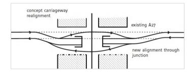
8.3.46 A further complication at Stockbridge is the proximity of the Chichester Canal being just over 200m from the junction. This could place some constraints on the vertical alignment through the junction that could require some variations in alignments of both the concept A27 underpass and the A286, and/or movement
